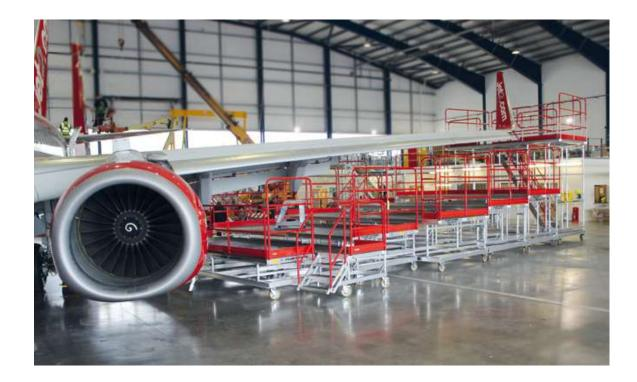
ound in both the commercial and military sectors our mobile aircraft access systems provide maintenance personnel the ideal platform to work at height safely. Manufactured from aluminium to offer a lightweight, strong and manoeuvrable system our designs cover access to all areas of the aircraft.
