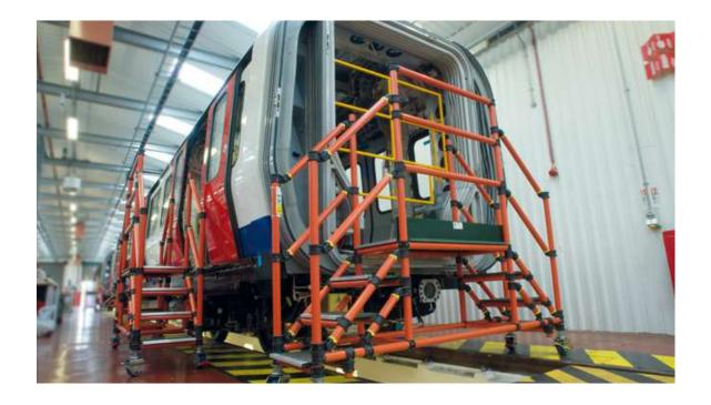
e offer tower systems, platforms and podiums to help with your every need. We developed Protec, our Glass Reinforced Plastic (GRP) solution for the ultimate in safety for work at height regulations.
